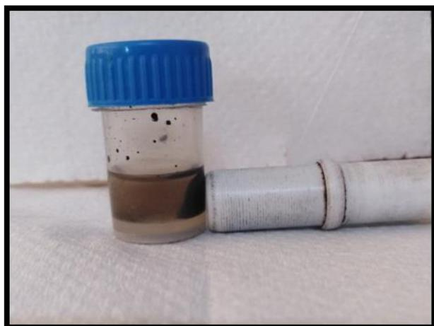
**Fig. 2** : Actual photographs of Fe<sub>3</sub>O<sub>4</sub> solution and magnetic attraction of Fe<sub>3</sub>O<sub>4</sub> nano-particles .
