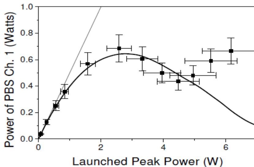
**Figure 3.:** Minimum output power of PBS channel 1 as a function of the launched power for a 200 m long PM fiber. Squares: measured data, solid curve: prediction from our model, straight line: prediction in the absence of
