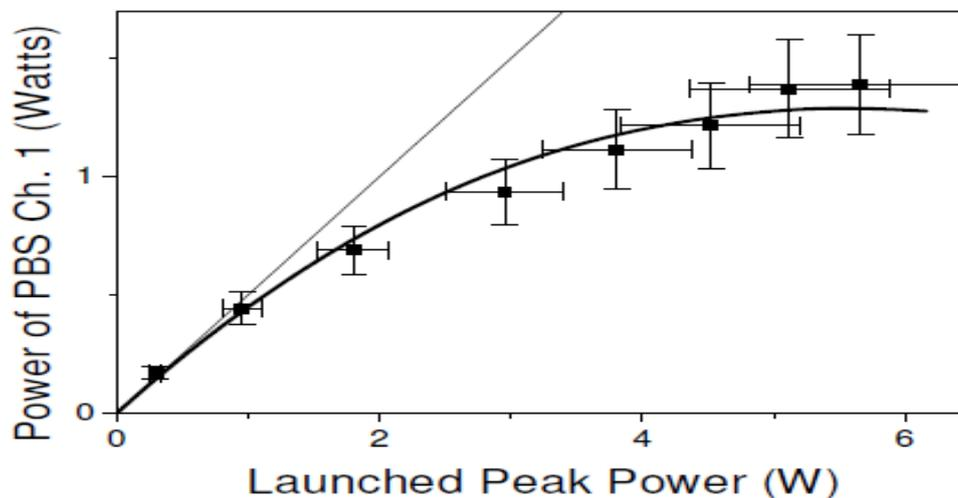
**Figure 4.:** Minimum output power of PBS channel 1 as a function of the launched power for a 100 m long PM fiber. Squares: measured data, solid curve: prediction from our model, straight line: prediction in the absence of NPR.
