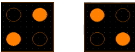
Figure 2: P = +1 Binary Logic 1 P = -1 Binary Logic 0
