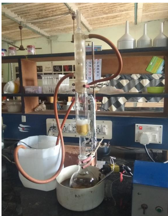
Fig-3. Soxhlet extraction of Alpinia galangal rhizome material
