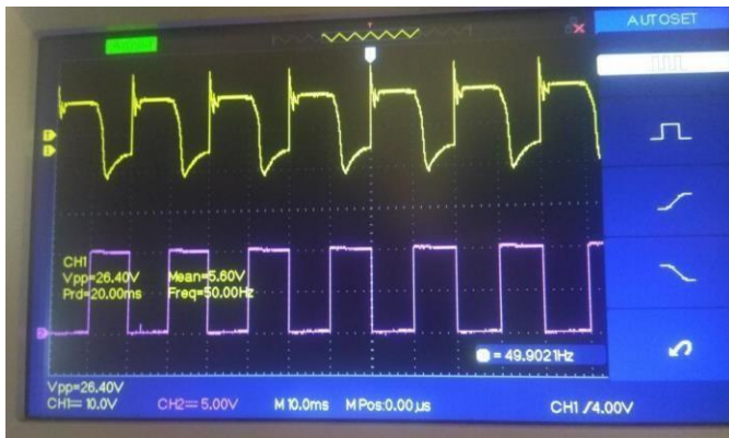
Fig 5.2: Single Phase Inverter Output Voltage Waveform In DSO.
