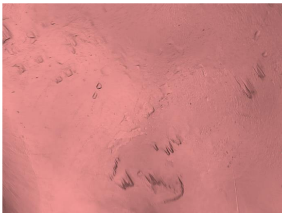
Figure 1. Surface of zinc bromide doped L-arginine monohydrate crystal before etching
