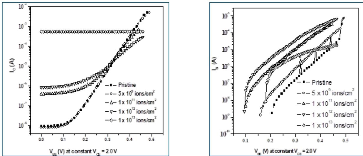
**Figure 3** Gummel plots ( $I_B$  and  $I_C$  Vs  $V_{BE}$ ) of 50 MeV  $\text{Li}^{3+}$  ion irradiated transistor 2N 3055 irradiated at room temperature (The results recorded at  $V_{CE} = 2.0$  V constant).
