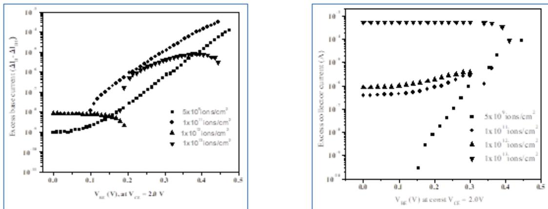
**Figure 2** Excess base and excess collector currents ( $\Delta I_B - \Delta I_{B0}$  and  $\Delta I_C - \Delta I_{C0}$  Vs  $V_{BE}$ ) of 50 MeV  $\text{Li}^{3+}$  ion irradiated transistor 2N 3055 irradiated at room temperature (The results recorded at  $V_{CE} = 2.0$  V constant).
