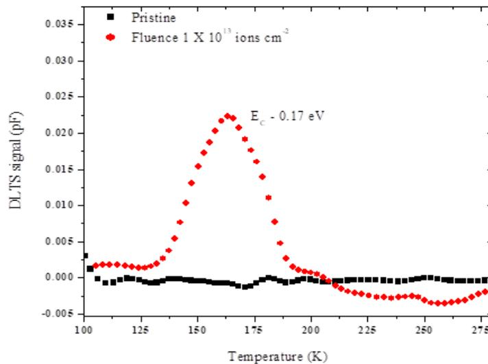
**Figure 5** DLTS spectra 50 MeV  $\text{Li}^{3+}$  ion irradiated 2N 3055 transistor for a fluence of  $1 \times 10^{13}$  ions/cm<sup>2</sup>
