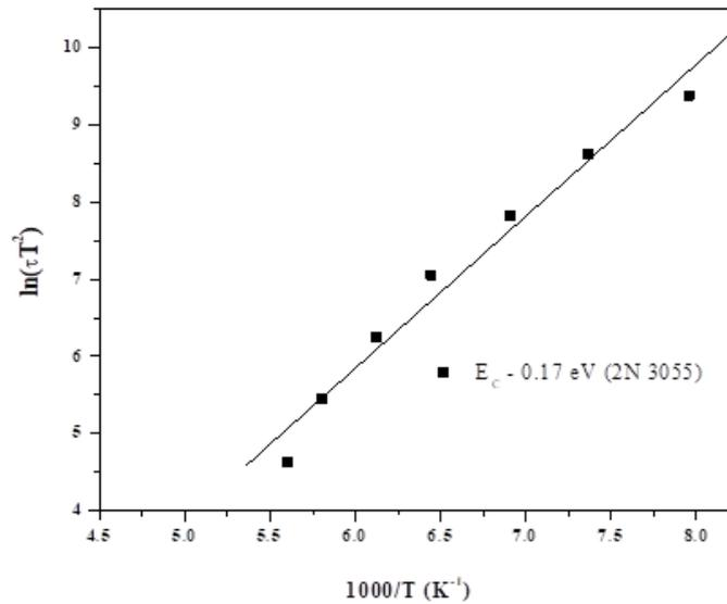
**Figure 6** Arrhenius plot for deep level defects for an ion fluence of  $1 \times 10^{13}$  ions/cm<sup>2</sup>.
