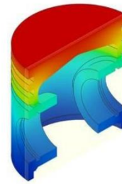
Fig -12: Cross Sectional view of temperature distribution (Al 6061)
