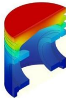
Fig -16: Cross Sectional view of temperature distribution (Titanium)
