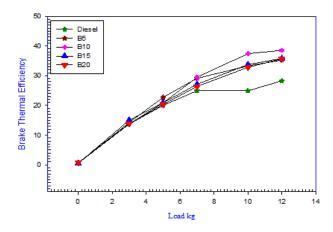
**Figure 6 :** Graph showing Brake Thermal Efficiency against different Loads (Kg) for pure diesel and combination of KOME blend
