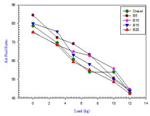
Figure 7: Graph showing Air Fuel Ratio against different Loads (Kg) for pure diesel and combination of KOME blend
