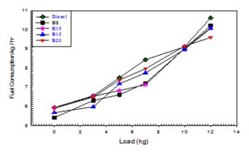
Figure 5: Graph showing Fuel Consumption (Kg/hr) against different Loads (Kg) for pure diesel and combination of KOME blend
