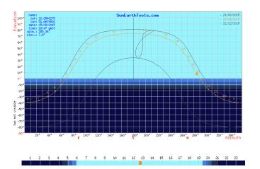
Figure 10: Sun position Diagram of Isfahan (sunearthtools.com, 2015)
