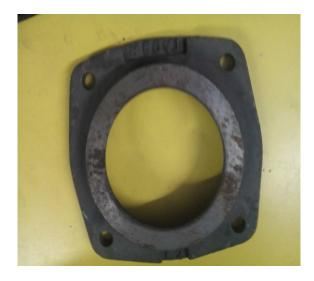
Figure 1 : Component with Shrinkage – Porosity defects
