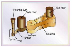
Figure 3: Parts of Typical Gating System
