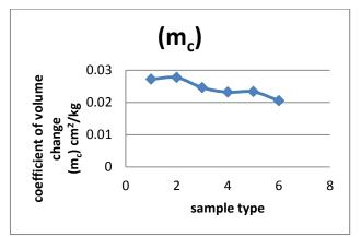
Graph-7: Variation of Coefficient of Volume Change for diiferent % of GGBS and Jute Fibre
