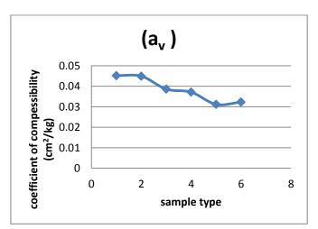
**Graph-5:** Variation of Coefficient of Compressibility for different % of GGBS and Jute Fibre
