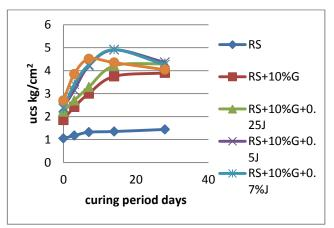
Graph-4: UCS variation at different curing periods at different % of Jute Fibre
