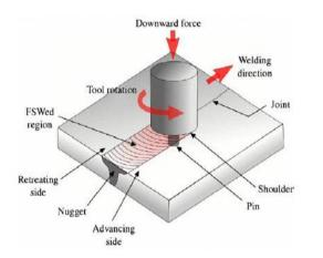
Figure 1 : Schematic diagram of friction stir welding process [6]
