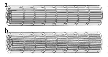
Fig. 2. (a) Rod-baffle heat exchanger with plain tubes.(b) Rod-baffle heat exchanger with spirally corrugated tubes.
