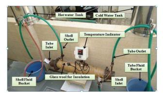
Fig 4. Photo of Experimental set up of STHX
