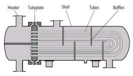
Fig 1- U tube heat exchanger
