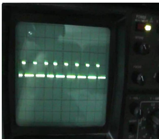
Figure 15a: PWM signal at duty cycle = 25% Horizontal: 2 msec/div. Vertical; 10 volt/div.
