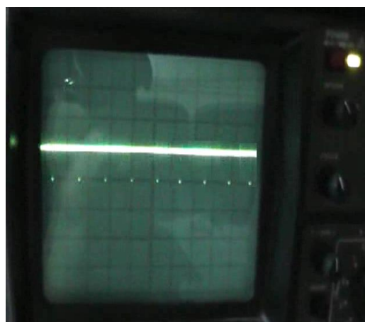
Figure 15d: PWM signal at duty cycle = 100% Horizontal: 2 msec/div. Vertical; 10 volt/div.
