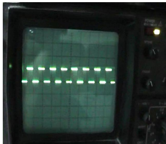
Figure 15b: PWM signal at duty cycle = 50% Horizontal: 2 msec/div. Vertical; 10 volt/div.
