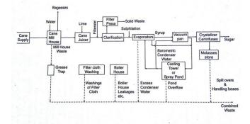
Figure 1: Flow Diagram for Sugar Manufacturing Process
