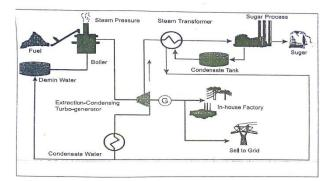
**Figure 3:** Process Flow Diagram for the Sugar Manufacturing Process of Industry.
