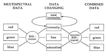
Figure 2. Principle of combination multisensor data
