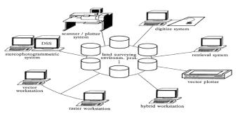
Figure 6. Decentralized hardware architecture including workstations
