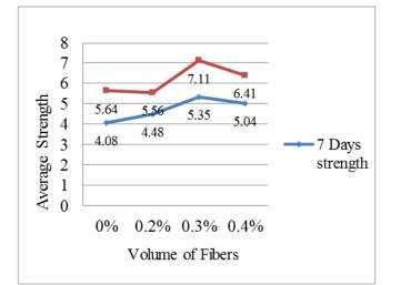
The graph shows that early strength is achieved by member having 0.3% vol. of polypropylene fiber. Member got maximum compressive strength by use of 0.3% of polypropylene fiber for 28 days.
