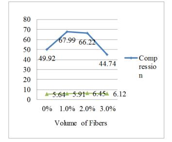
Strength analysis of Steel Fiber Reinforced Concrete for 28 days
