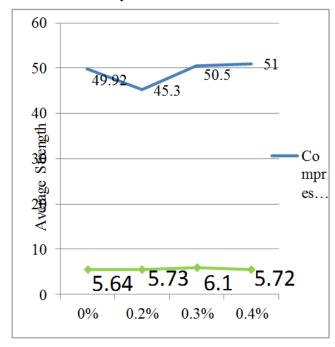
The graph shows that how all the 28 days strengths vary by changing percentage of synthetic fibers. We can say that flexure strength increases up to 0.3% of volume of fibers but beyond that it decreases. Compressive strength increases after 0.3% of volume of fibers
