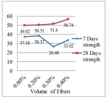
The graph shows that early strength is achieved by member having 0.2% vol.ofpolypropylene fiber. Member got maximum compressive strength by use of 0.4% of polypropylene fiber for 28 days.
