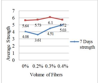
The graph shows that early strength is achieved by member having 0.4% vol. of synthetic fiber. Member got maximum compressive strength by use of 0.3% of synthetic fiber for 28 days.
