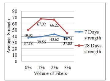
The graph shows that early strength is achieved by member having 2% vol. of steel fiber. Member got maximum compressive strength by use of 1% of steel fiber for 28 days
