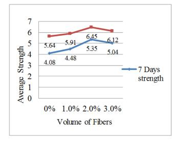
Flexural strength analysis of SF concrete
