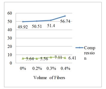
The graph shows that how all the 28 days strengths vary by changing percentage of polypropylene fibers.We can say that flexure strength doesn't vary that much but Compressive strength is considerably increased at 0.4%
