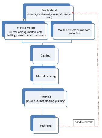
Figure 1 : Flow Diagram for Casting Manufacturing Process.
