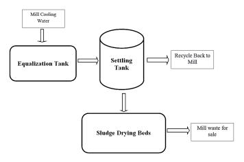
Figure 2 : Process Flow Diagram of ETP of Industry
