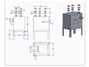
Figure 2. sketch of multistage three roller pipe bending machine
