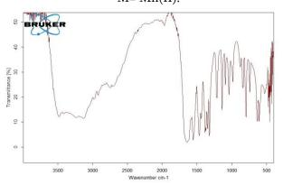
**Figure 3.** FT-IR Spectrum of Mn(II) complex of 2-hydroxy-6-methylnicotinic acid
