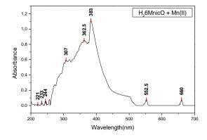
**Figure 4.** UV-Visible spectrum of Mn(II) complex of 2-hydroxy-6-methylnicotinic acid
