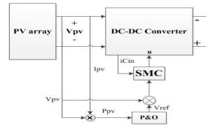
Figure 4.smc design based on voltage error and input capacitive current block diagram
