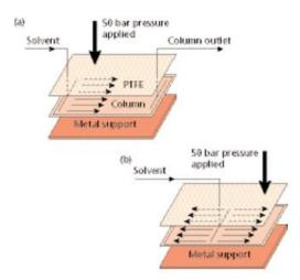
**Figure 3:** OPLC cassette design for (a) linear onedimensional and (b) bidirectional chromatography separations steps.
