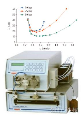
**Figure 2:** Plate height versus linear flow velocity as a function of applied pressure in OPLC for HPTLC layers (5-mm particle size) b) Instrument of OPLC
