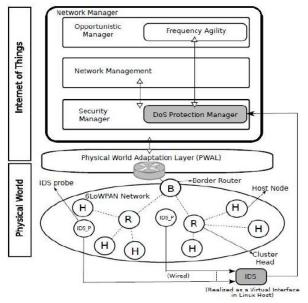
Figure 1. DoS Detection Architecture
