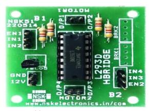
Figure 4 (a). Motor driver circuit of H-bridge
