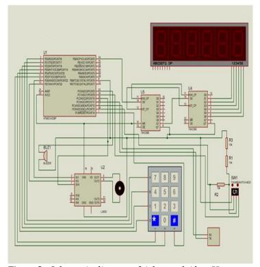
**Figure 2.** Schematic diagram of Advanced Alert Home locker security systemwit Fingerprint and Soft password with Audrina Uno
