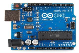
Figure 7. Arduino UNO board
