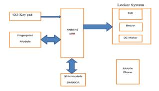
**Figure 1.** Block diagram of Advanced Alert Home locker security system.
