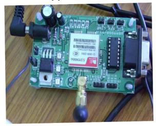
Figure 6. GSM SIM900 Circuit
