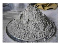
Ground Granulated Blast Furnace Slag (GGBS) is a waste product from the blast furnaces used to make iron. These functions at a temperature of about 1500 degrees centigrade and are discontented with a carefully controlled mixture of iron ore, coke and limestone.
