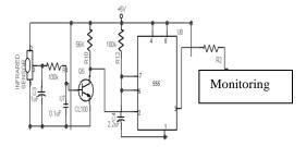
**Figure 2**. Pulse rate Detection Circuit
