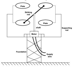
Figure 1. mechanism of sounding bell
