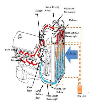
An engine, two radiators- one conventional and another fabricated with twisted tubes, nanofluid (SiO2), venturimeter, thermometer.
