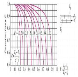
7. Area of the heat transfer after considering correction factor is given as,
