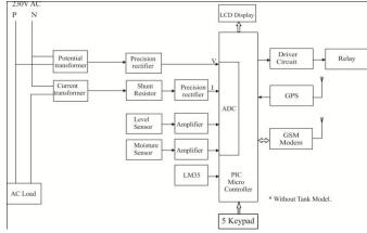
Figure 1. Block Diagram Of Proposed System
