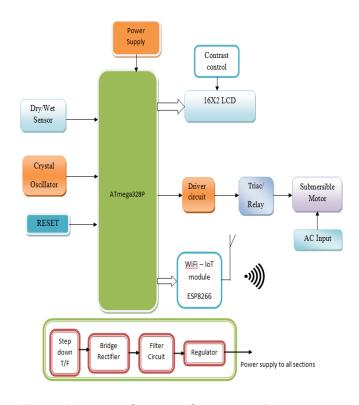
Figure 1. Proposed Iot Based Irrigation System.
