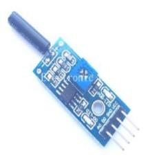
Figure 6. Vibration Sensor
