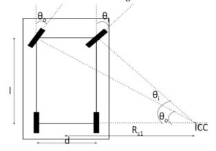
In fig. θo= Angle of outside Lock θi= Angle of Inside Lock d= Wheel Track l= Wheel Base
