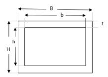
Considering Rectangular cross section of material Bending stress =M/Z  $Z=BH^2/6 - bh^3/6H$ B=1.5"=38.1mmH=1"=25.4mmThickness (t) =2mm b=34.1mmh=21.4mm $Z=38.12\times5.4^2/6 - 34.12\times1.4^3/6\times25.4$  $= 2\times10^3 \text{ mm}^3$
