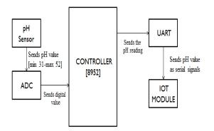
Figure 1. Workflow of the system
