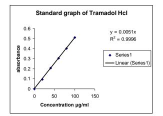
Figure 1. Estimation of Tramadol Hcl, measured at 271 nm using UV Spectrophotometer
