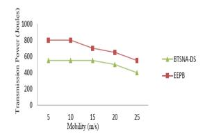
**Figure 10.** Transmission Power (Joules) Vs. Mobility (m/s).
