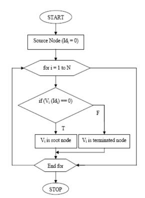
Figure 4. Root Node Construction for BTSNA-DS.
