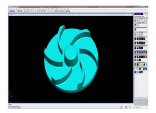
Figure 2. CAD model of the pump impeller
