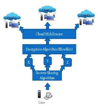
**Figure 2.** Proposed Architecture for Cloud Computing
