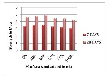
**Chart -2:** Difference of 7 days and 28 days Flexural strength test results
