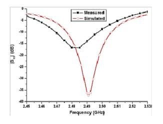
Figure 4. S11 for the proposed antenna
