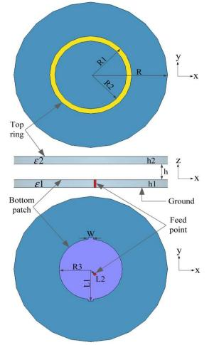
Figure 1. Geometry of the wide-beam circularly-polarized microstrip antenna
