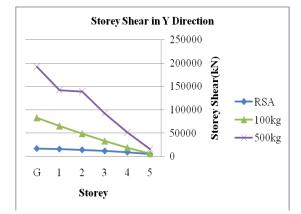
Figure 5: Storey shear profile in transverse direction
