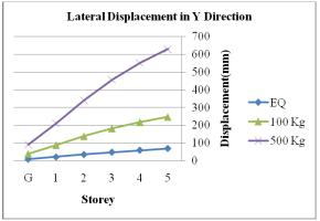
Figure 4: Displacement profile in transverse direction
