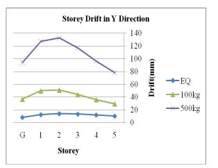
Figure 4.26: Drift profile in transverse direction
