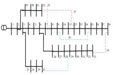
Figure 2: single line diagram of 33bus test system
