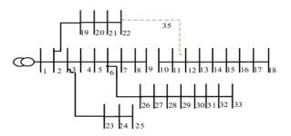
**Figure 3** : single line diagram of 33bus test system after reconfiguration
