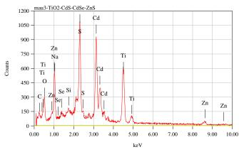
**Figure 2.** (a) The SEM image and (b) the EDS of the TiO<sub>2</sub>/CdS/CdSe/ZnS photoanode.
