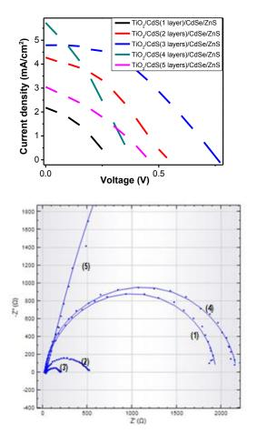
**Figure 4.** (a) The I-V curves and (b) the Nyquist plots of the QDSSCs with the different photoanodes.
