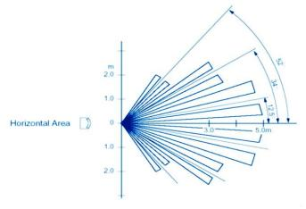
Figure 2: Pyroelectric sensor field of view
