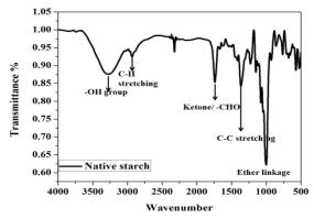
Figure 1. FTIR spectra of starch
