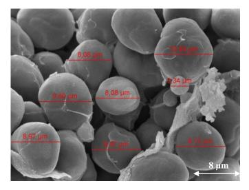
Figure 1b: SEM-picture from maize 'M\_008' (x 3000)
