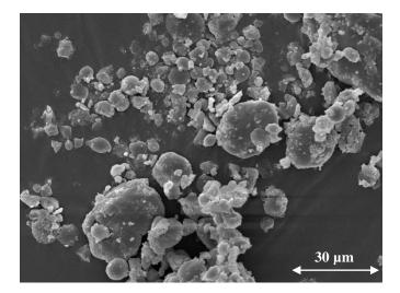
Figure 2a: SEM-picture from oat grains 'Melody' (x 1000)
