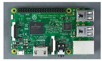
Figure 4. Raspberry pi 3 model b
