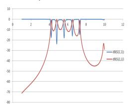
Fig.3: S11 and S21 plot with U-Shaped DGS
