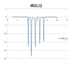
Fig.4: S11 plot with U-Shaped DGS
