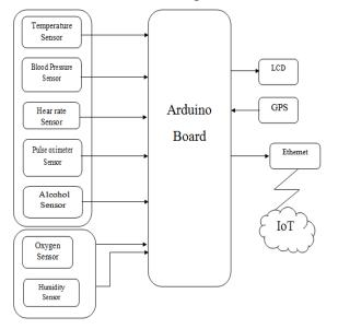
Figure 1: Block Diagram
