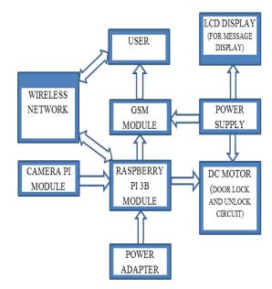
**Figure 1.** block diagram of "achieving advance security system over raspberry pi controlled via android application".
